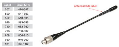
NOTE: with increasing frequency the length of the antenna decreases (therefore use short antenna for high frequencies, long antenna for low frequencies)
